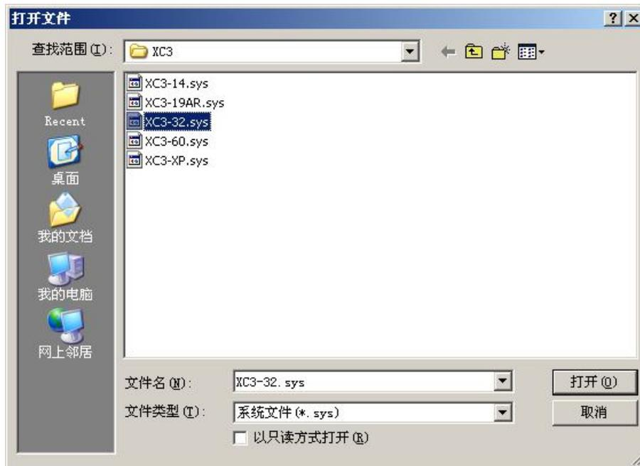
**Note:**No 24, 48 points PLC in the list, so take XC-32,60 points instead of XC-24,48. It should be note that after upgrade, in the XCP software, you should choose XC3-32, 60, not XC3-24,48! However, the function will be still XC3-24,48!
